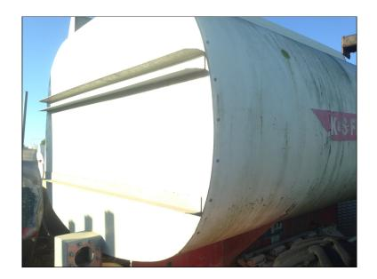
ALLOY FUEL TANKS WITH STEEL ENDS APPROXIMATELY: 10,000 - 16,000 LITRES
